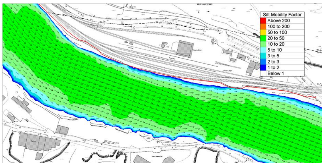
Plate 7.2 Fine silt mobility factor at mid-ebb spring tide – proposed case (Hydro Environmental Ltd., 2021).
